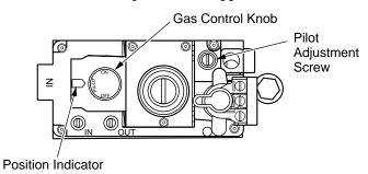
Figure 39 - Control Knob in the PILOT position
